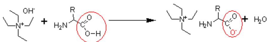
Scheme 9: Deprotonation of carboxylic acid residue by hydroxide ion to form carboxylate ion and water as by-product.
