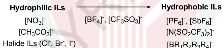
Figure 2.7. Different types of anions responsible for water miscibility and immiscibility of ILs.
