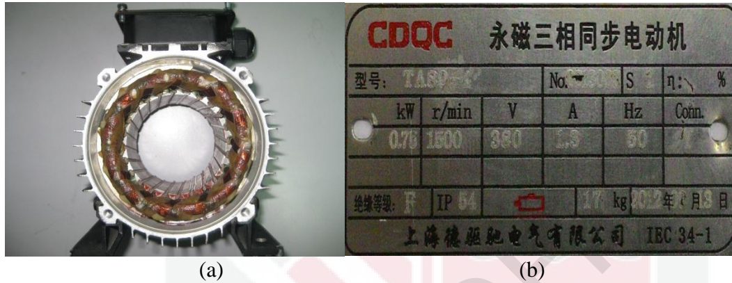
Figure 3.7: (a) LS-PMSM used in this research and (b) its nameplate
